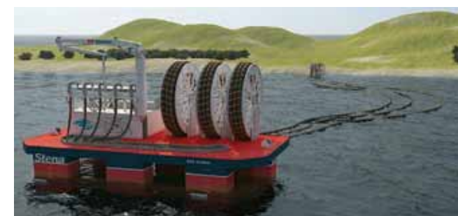
Photo: Stena The JFT unit contains all the required equipment, systems and safety features normally installed on a jetty.
